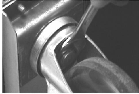
**TIGHTEN CASTER WITH 18 mm OPEN END WRENCH**
