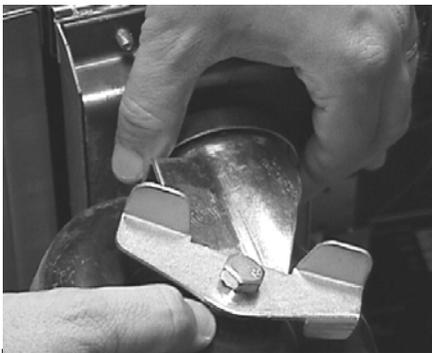
**INSTALLING CASTER INTO LEG SUPPORT ASSEMBLY**
